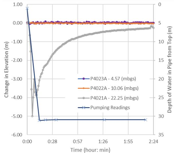
Figure 7. I4020 Vibrating Wire Piezometer Responses to Pumping of the SI Casing
