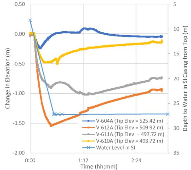
Figure 10. I-63 Vibrating Wire Piezometer Responses to Pumping of the SI Casing
