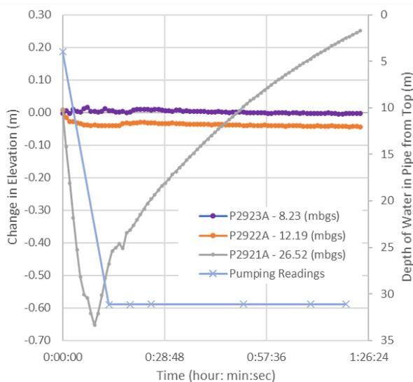
Figure 6. I2920 Vibrating Wire Piezometer Responses to Pumping of the SI Casing
