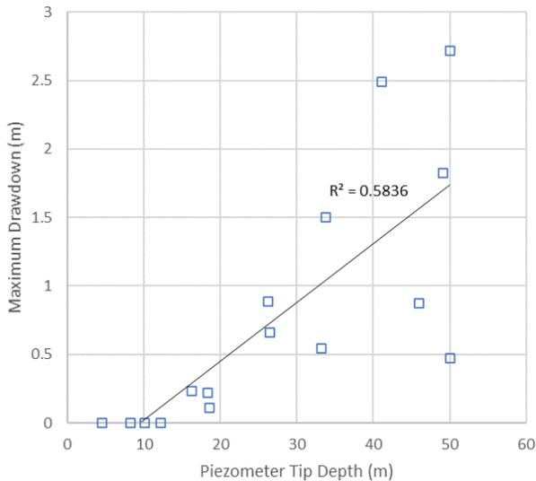
Figure 12. Tip Depth versus Maximum Observed Drawdown Excluding Outlier
