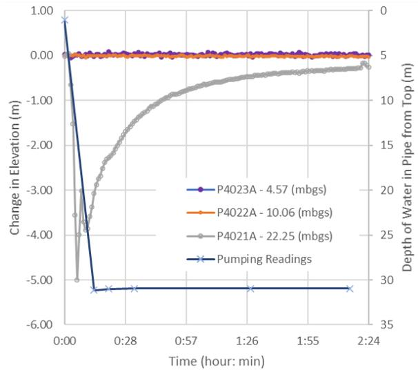
Figure 7. I4020 Vibrating Wire Piezometer Responses to Pumping of the SI Casing
