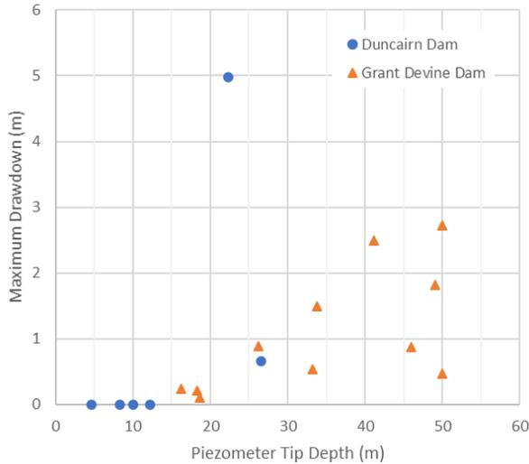
Figure 11. Tip Depth versus Maximum Observed Drawdown
