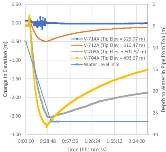
Figure 9. I-73 Vibrating Wire Piezometer Responses to Pumping of the SI Casing
