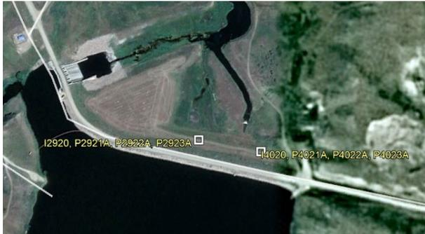
Figure 3. Duncairn Dam layout and instrument locations (modified from Google Earth, 2021).
