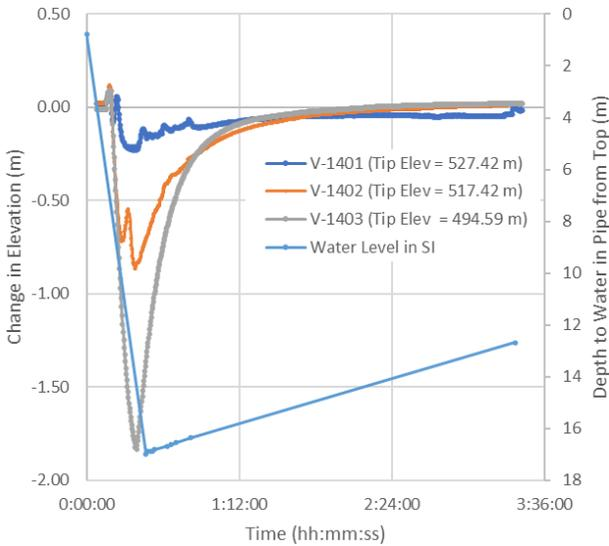
Figure 8. I-141 Vibrating Wire Piezometer Responses to Pumping of the SI Casing
